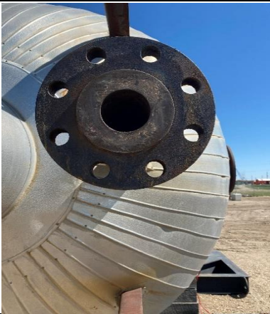
Photo 6: 4" top flange in good condition
