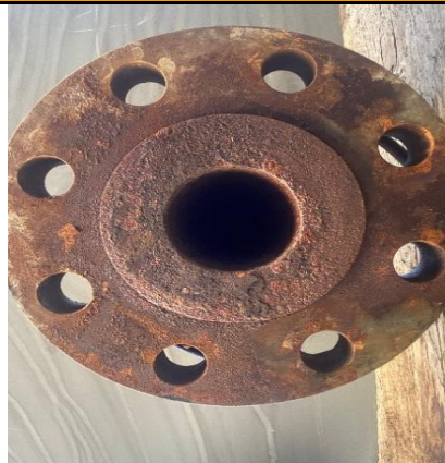
Photo 8: 4" Bottom Flange where damage is present
